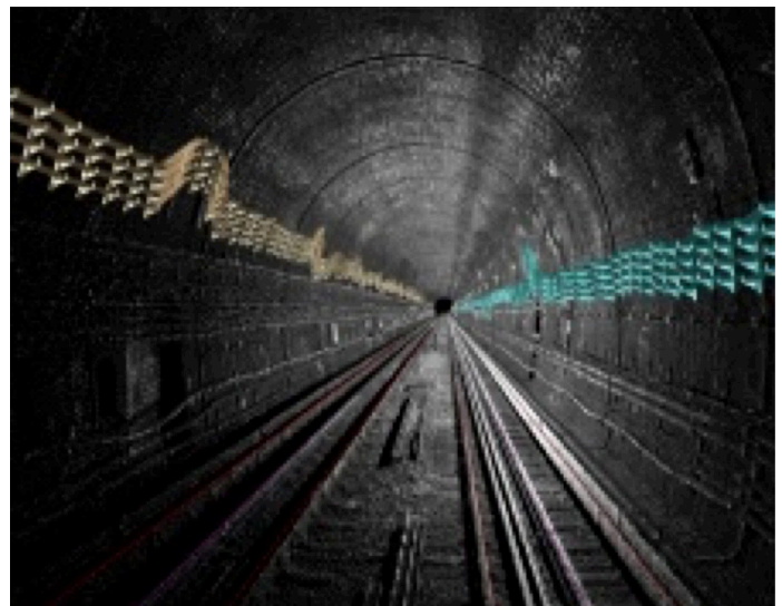
Suggested cable design plot, based on the “shortest path” method.
